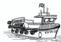
This is an example of a **creel boat**; when setting, checking or collecting creels, the vessel may be stationary for several minutes, then move off quickly. Often they can be seen working very close to the shore in rocky areas. Usually fluorescent marker buoys will be seen in the water near these boats.
